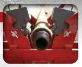
Auto index device is designed to feed one pipe at a time.
