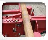
Hydraulic racks stow on the loader for ease of transport. Racks can be positioned to load pipe from either side.
